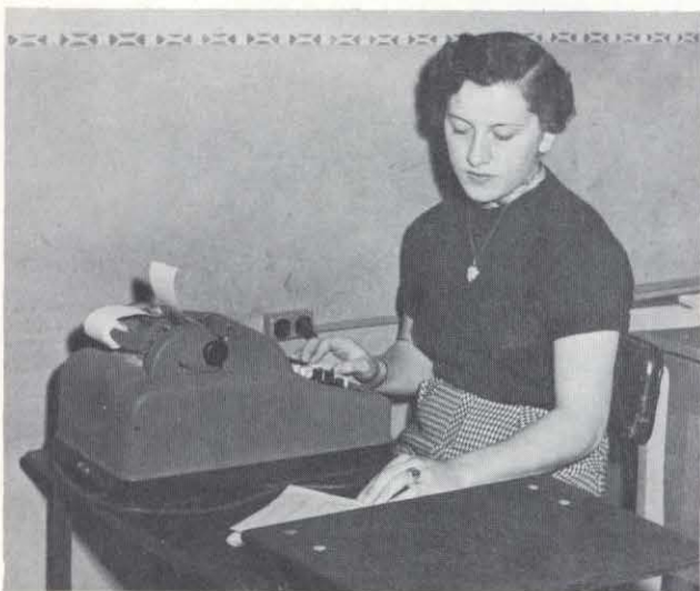
It might have only ten keys, but the operation of this ten-key adding machine still takes a while to learn. The reason is that on the ten-key you can add, divide, multiply and subtract.
